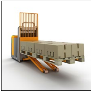
Scissor lift for order picking at an ergonomic height
