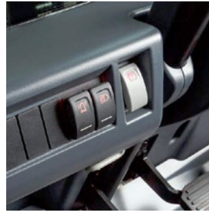
Electrically applied parking brake, easily operated at the push of a button.
