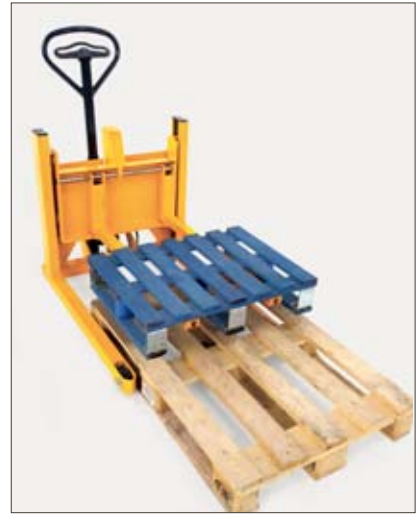
A half pallet is picked up from a standard Euro pallet
